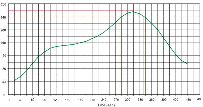
Peak Temp=257°C, Ramp Rate=0.802deg. °C/sec
