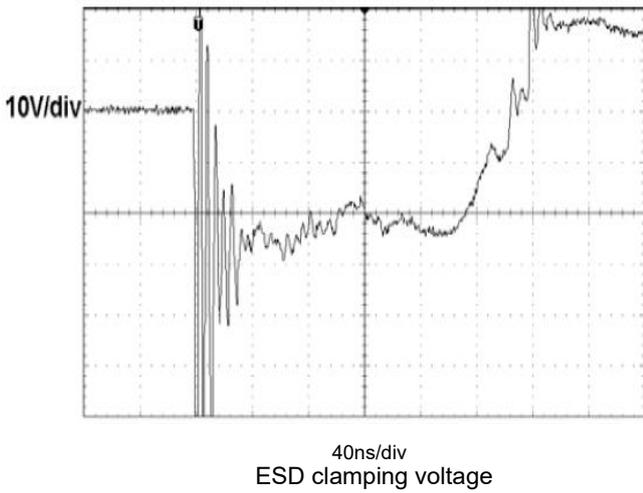
Fig 9. (IEC61000-4-2-8KV contact)
