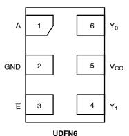
Figure 1. Pinout (Top View)
