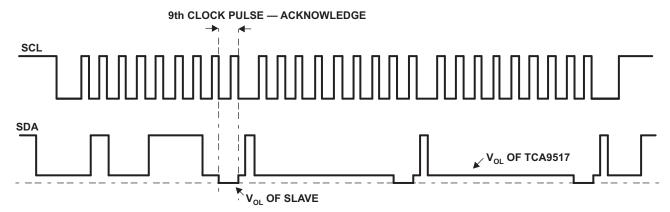
Figure 11. Bus B (2.7 V to 5.5 V Bus) Waveform
