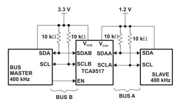
Figure 7. Typical Application Schematic
