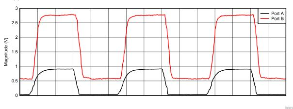
Figure 12. Voltage Translation at 400 kHz,  $V_{CCA} = 0.9 \text{ V}$ ,  $V_{CCB} = 2.7 \text{ V}$
