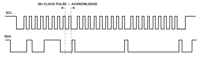
Figure 10. Bus A (0.9 V to 5.5 V Bus) Waveform
