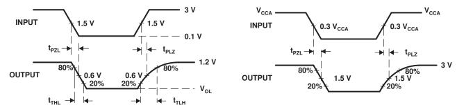
Figure 4. Waveform 1 – Propagation Delay and Transition Times for B-side to A-side
