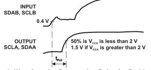
Figure 6. Waveform 3 - Propagation Delay for B-side to A-side
