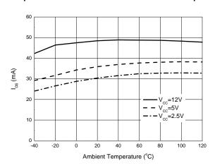
**Supply Current vs. Ambient Temperature**
