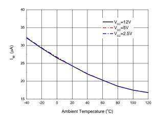
**Output Short Circuit Current vs. Ambient Temperature**
