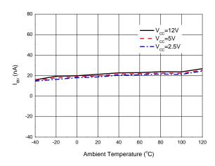
I<sub>CTRL</sub> Pin Input Bias Current vs. Ambient Temperature
