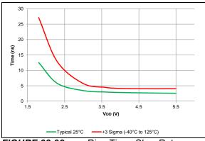
FIGURE 38-98: Rise Time, Slew Rate Control Disabled.
