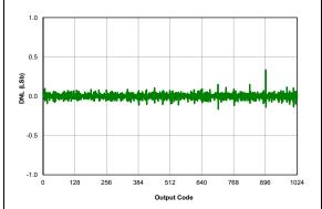
**FIGURE 38-46:** ADC, DNL, VDD = 3.0V,  $TAD = 4 \mu S$ ,  $25^{\circ}$ C.
