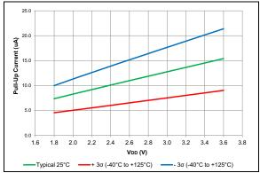
FIGURE 38-102: Weak Pull-up Current, PIC16LF18855/75 Only.
