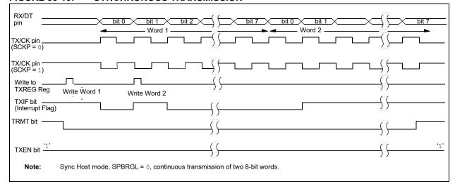
FIGURE 33-11: SYNCHRONOUS TRANSMISSION (THROUGH TXEN)
