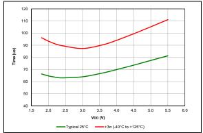
FIGURE 38-42: Wake From Sleep, VREGPM = 1, HFINTOSC = 16 MHz, PIC16F18855/75 Only.
