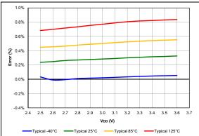
**FIGURE 38-87:** FVR Voltage Error 2x, PIC16LF18855/75 Only.
