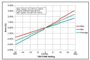
FIGURE 38-100: OSCTUNE Center Frequency, PIC16LF18855/75 Only.
