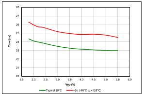
FIGURE 38-41: Wake From Sleep, VREGPM = 0, HFINTOSC = 16 MHz, PIC16F18855/75 Only.
