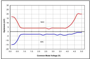
FIGURE 38-66: Comparator Offset, NP Mode (CxSP = 1), VDD = 5.0V, Typical Measured Values at 25°C, PIC16F18855/75 Only.
