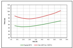
FIGURE 38-40: Wake From Sleep, VREGPM = 1, HFINTOSC = 4 MHz, PIC16F18855/75 Only.
