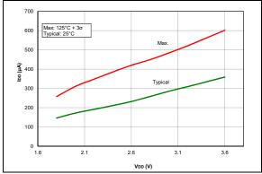
FIGURE 38-10: IDD, ECM Oscillator, Fosc = 4 MHz, PIC16LF18855/75 Only.
