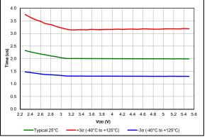
**FIGURE 38-76:** ADC RC Oscillator Period, PIC16F18855/75 Only.
