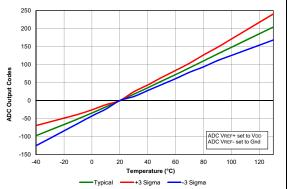
FIGURE 38-58: Temp. Indicator Slope Normalized to 20°C, High Range, VDD = 3.0V.
