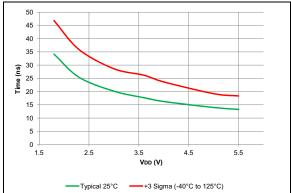
FIGURE 38-96: Rise Time, Slew Rate Control Enabled.
