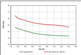
FIGURE 38-39: Wake From Sleep, VREGPM = 0, HFINTOSC = 4 MHz, PIC16F18855/75 Only.
