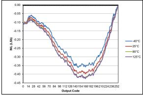
FIGURE 38-71: Typical DAC INL Error, VDD = 3.0V, VREF = External 3V.
