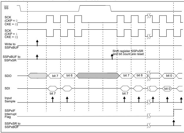
FIGURE 31-9: SPI MODE WAVEFORM (CLIENT MODE WITH CKE = 0)
