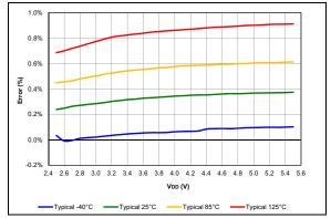
**FIGURE 38-88:** FVR Voltage Error 2x, PIC16F18855/75 Only.
