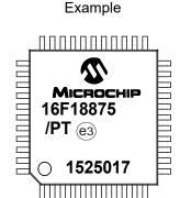
44-Lead QFN (8x8x0.9 mm)
