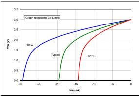
FIGURE 38-15: VOH vs. IOH Over Temperature, VDD = 3.0V.
