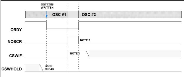
Note 1: CSWIF is asserted coincident with NOSCR; interrupt is serviced at OSC#2 speed.
