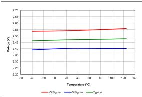
FIGURE 38-27: Brown-Out Reset Voltage, Trip Point (BORV = 1x).
