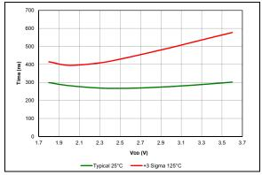
**FIGURE 38-82:** Comparator Response Time, Rising Edge, PIC16LF18855/75 Only.
