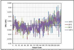
FIGURE 38-70: Typical DAC DNL Error, VDD = 3.0V, VREF = External 3V.
