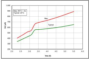
FIGURE 38-4: IDD, ECM Oscillator, Fosc = 4 MHz, PIC16F18855/75 Only.
