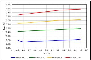
FIGURE 38-85: Typical FVR Voltage 1x, PIC16LF18855/75 Only.
