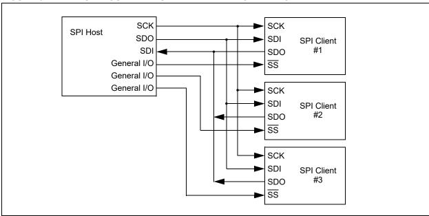
FIGURE 31-4: SPI HOST AND MULTIPLE CLIENT CONNECTION
