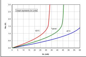
FIGURE 38-16: VOL vs. IOL Over Temperature, VDD = 3.0V.
