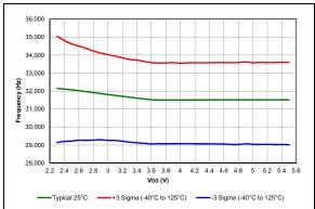
FIGURE 38-20: LFINTOSC Frequency, PIC16F18855/75 Only.
