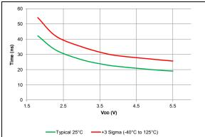
**FIGURE 38-97:** Fall Time, Slew Rate Control Enabled.
