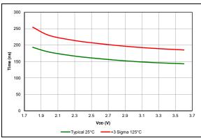
FIGURE 38-80: Comparator Response Time, Falling Edge, PIC16LF18855/75 Only.
