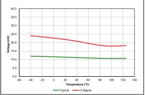
FIGURE 38-28: Brown-Out Reset Hysteresis, Trip Point (BORV = 1x).
