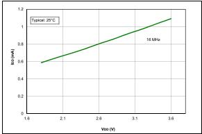
FIGURE 38-11: IDD, ECH Oscillator, Typical, PIC16LF18855/75 Only.
