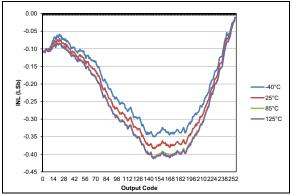
**FIGURE 38-73:** Typical DAC INL Error, VDD = 5.0V, VREF = External 5V, PIC16F18855/75 Only.
