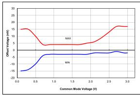
FIGURE 38-63: Comparator Offset, NP Mode (CxSP = 1), VDD = 3.0V, Typical Measured Values at 25°C.
