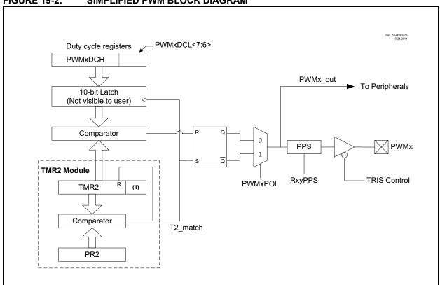
Note 1: 8-bit timer is concatenated with two bits generated by Fosc or two bits of the internal prescaler to
