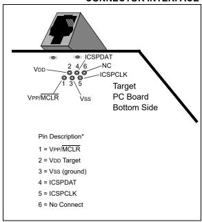
Another connector often found in use with the PICkit™ programmers is a standard 6-pin header with 0.1 inch spacing. Refer to Figure 35-2.
