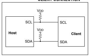
The Acknowledge bit  $(\overline{ACK})$  is an active-low signal, which holds the SDA line low to indicate to the transmitter that the client device has received the transmitted data and is ready to receive more.
