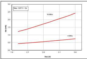
FIGURE 38-9: IDD Maximum, INT Oscillator, PIC16LF18855/75 Only.
