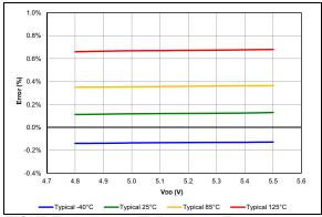
**FIGURE 38-89:** FVR Voltage Error 4x, PIC16F18855/75 Only.
