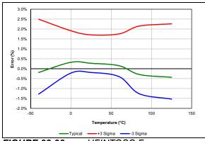
FIGURE 38-92: HFINTOSC Frequency Error, VDD = 3.0V.
