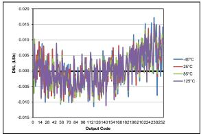
**FIGURE 38-72:** Typical DAC DNL Error, VDD = 5.0V, VREF = External 5V, PIC16F18855/75 Only.
