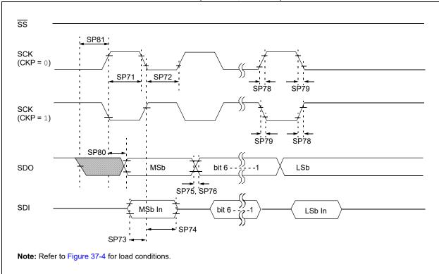
FIGURE 37-18: SPI HOST MODE TIMING (CKE = 1, SMP = 1)
