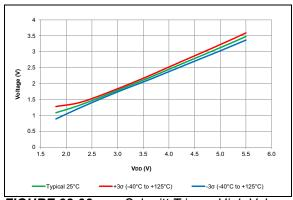
FIGURE 38-93: Schmitt Trigger High Values.
