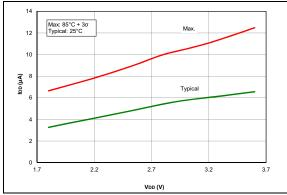
**FIGURE 38-7:** IDD, LFINT, Fosc = 31 kHz, PIC16LF18855/75 Only.
