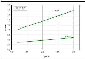
FIGURE 38-8: IDD Typical, INT Oscillator, PIC16LF18855/75 Only.
