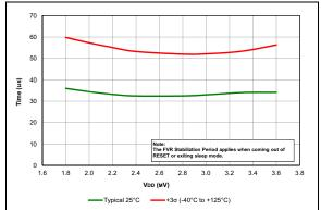
FIGURE 38-84: FVR Stabilization Period, PIC16LF18855/75 Only.
