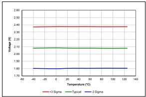
**FIGURE 38-31:** LPBOR Reset Voltage, PIC16LF18855/75 Only.
