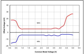
FIGURE 38-67: Comparator Offset, NP Mode (CxSP = 1), VDD = 5.5V, Typical Measured Values from -40°C to 125°C, PIC16F18855/75 Only.
