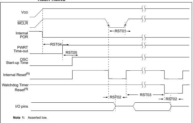
FIGURE 37-9: BROWN-OUT RESET TIMING AND CHARACTERISTICS
