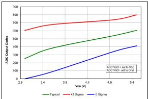
FIGURE 38-53: Temp. Indicator Initial Offset, High Range, Temp. = 20°C, PIC16F18855/75 Only.
