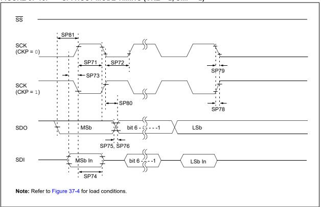
FIGURE 37-19: SPI CLIENT MODE TIMING (CKE = 0)
