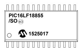
28-Lead SSOP (5.30 mm)
