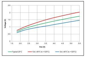
FIGURE 38-94: Schmitt Trigger Low Values.
