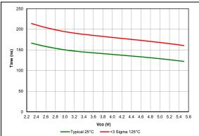
FIGURE 38-81: Comparator Response Time, Falling Edge, PIC16F18855/75 Only.
