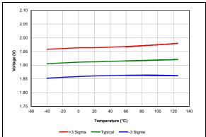
FIGURE 38-29: Brown-Out Reset Voltage, Trip Point (BORV = 11).
