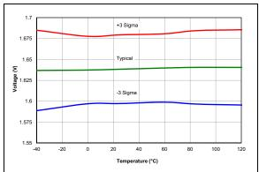
FIGURE 38-35: POR Release Voltage.
