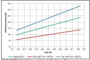
FIGURE 38-101: Weak Pull-up Current, PIC16F18855/75 Only.
