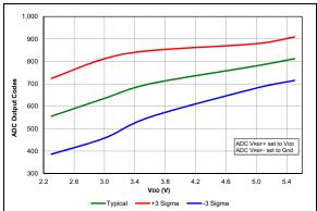
FIGURE 38-54: Temp. Indicator Initial Offset, Low Range, Temp. = 20°C, PIC16F18855/75 Only.
