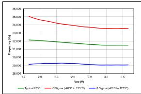
FIGURE 38-19: LFINTOSC Frequency, PIC16LF18855/75 Only.
