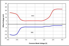
FIGURE 38-64: Comparator Offset, NP Mode (CxSP = 1), VDD = 3.0V, Typical Measured Values from -40°C to 125°C.
