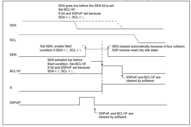
FIGURE 31-34: BUS COLLISION DURING START CONDITION (SCL = 0)
