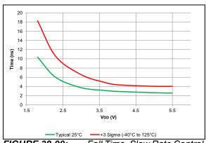
FIGURE 38-99: Fall Time, Slew Rate Control Disabled.
