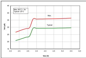
**FIGURE 38-1:** IDD, LFINT, Fosc = 31 kHz, PIC16F18855/75 Only.
