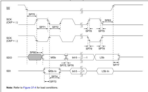
FIGURE 37-20: SPI CLIENT MODE TIMING (CKE = 1)
