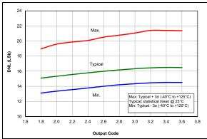
FIGURE 38-74: DAC INL Error, VDD = 3.0V, PIC16LF18855/75 Only.
