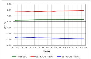
FIGURE 38-91: HFINTOSC Typical Frequency Error, PIC16F18855/75 Only.
