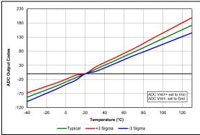
FIGURE 38-57: Temp. Indicator Slope
