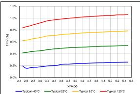
**FIGURE 38-86:** FVR Voltage Error 1x, PIC16F18855/75 Only.
