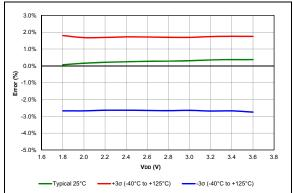
FIGURE 38-90: HFINTOSC Typical Frequency Error, PIC16LF18855/75 Only.
