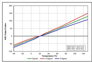
FIGURE 38-61: Temp. Indicator Slope Normalized to 20°C, Low Range, VDD = 2.3V.
