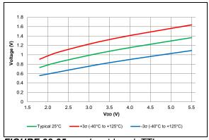
FIGURE 38-95: Input Level, TTL.
