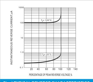
Fig.4 TYPICAL REVERSE CHARACTERISTICS
