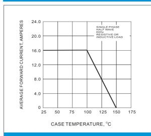
Fig.1 FORWARD CURRENT DERATING CURVE
