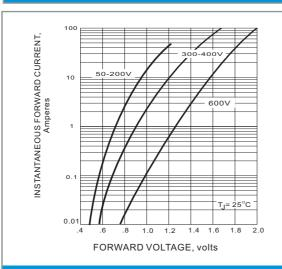
Fig.3 FORWARD CHARACTERISTICS
