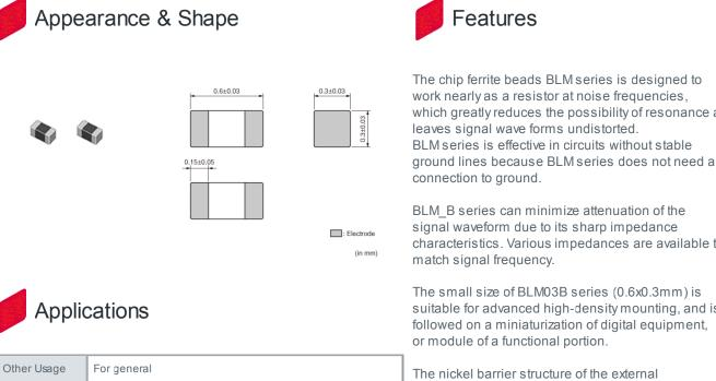
The chip ferrite beads BLM series is designed to work nearly as a resistor at noise frequencies, which greatly reduces the possibility of resonance and leaves signal wave forms undistorted. BLM series is effective in circuits without stable
