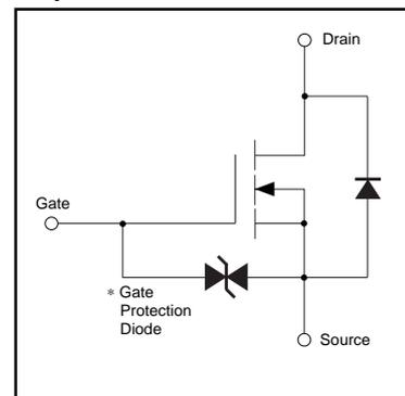
\*A protection diode is included between the gate and the source terminals to protect the diode against static electricity when the product is in use. Use a protection circuit when the fixed voltages are exceeded.
