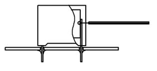
Temperature monitored inside the capacitor.
