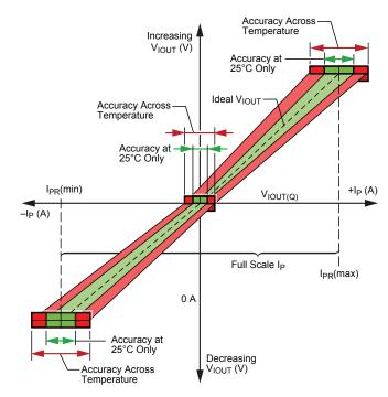
Figure 1: Output Voltage versus Sensed Current
