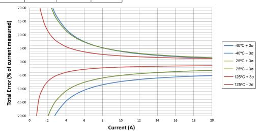
Figure 3: Predicted Total Error as a Function of the Sensed Current for the ACS730KLCTR-20AB
