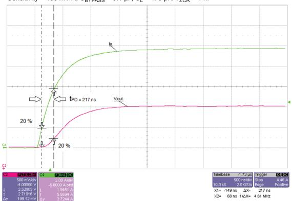
Rise Time ( $t_{RISE}$ ) 10 A input signal ( $I_P$ ) with rise time < 1  $\mu s$ Sensitivity = 100 mV/A,  $C_{BYPASS}$  = 0.1  $\mu F$ ,  $C_L$  = 470 pF,  $V_{ZCR}$  = 1 nF
