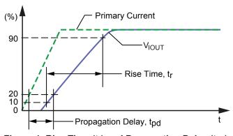
Figure 4: Rise Time (t<sub>r</sub>) and Propagation Delay (t<sub>pd</sub>)
