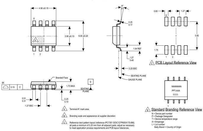
Figure 6: Package LC, 8-Pin SOICN
