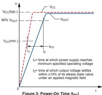
Figure 3: Power-On Time (t<sub>PO</sub>)
