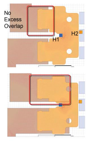
Figure 5: Simulations of ACS781 Leadframe with Different Overlap of the Current Trace and the I<sub>P</sub> Bus
