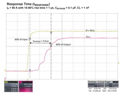
Rise Time ( $t_r$ ) I<sub>P</sub> = 90 A with 10%-90% rise time = 1 µs, C<sub>BYPASS</sub> = 0.1 µF, C<sub>L</sub> = 1 nF
