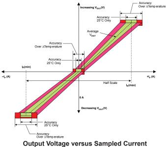
Total Output Error at 0 A and at Full-Scale Current
