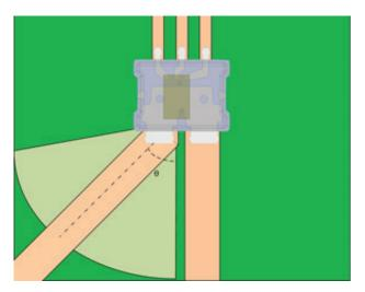
Figure 4: ACS781 Current Trace Approach – the desired range of the angle θ is from 0° to 85°
