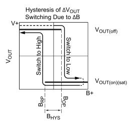
Figure 3: Output Voltage Responds to Magnetic Flux Density.
