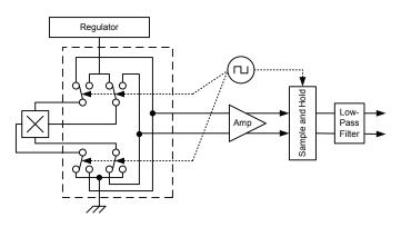
Figure 2: Chopper Stabilization Circuit (Dynamic Quadrature Offset Cancellation)
