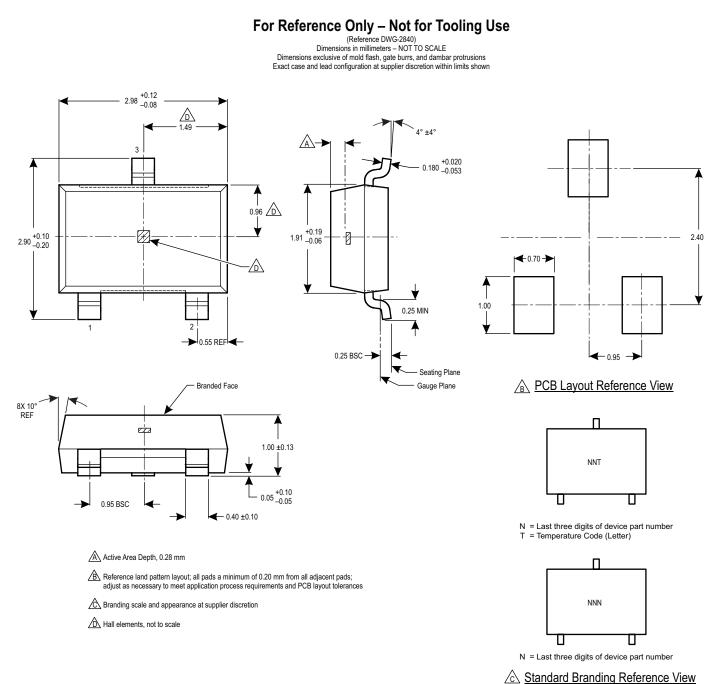
Figure 5: Package LH, 3-Pin SOT23W
