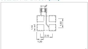
To ensure optimal oscillator performance, place a by-pass capacitor of 0.1µF as close to the part as possible between Vdd and GND pads.
