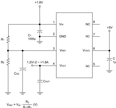
$$V_{REF} = V_{IN} \cdot \frac{R_2}{R_1 + R_2} (V)$$
