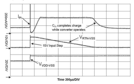
Figure 18. Response to PSE Step Voltage
