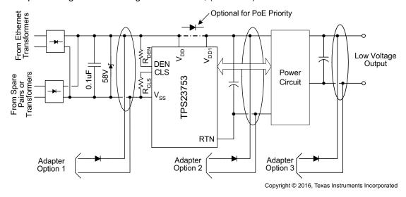
Figure 22. ORing Configurations
