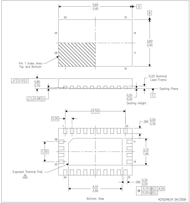
NOTES: A. All linear dimensions are in millimeters. Dimensioning and tolerancing per ASME Y14.5M—1994.
