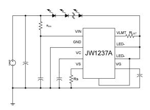
1. Because of the 30V zener integrated and the 16V  $V_{IN}$  start threshold, the value of  $R_{VIN}$  may satisfy the following conditions:
