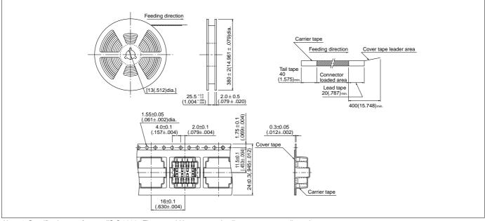
Note: 1. Specifications conform to JIS C 0806. The tape width, connector loading recess square dimensions, etc.are determined by the number of circuits and external shape of the connector to be loaded.
