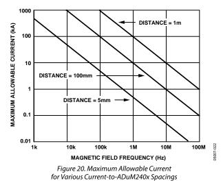
Note that at combinations of strong magnetic field and high frequency, any loops formed by printed circuit board traces could induce sufficiently large error voltages to trigger the thresholds of succeeding circuitry. Care should be taken in the layout of such traces to avoid this possibility.
