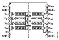
Figure 1. ADuM2400 Functional Block Diagram
