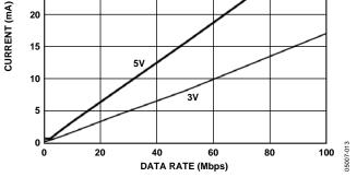
Figure 13. Typical ADuM2401  $V_{DD1}$  Supply Current vs. Data Rate for 5 V and 3 V Operation
