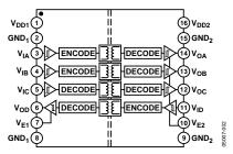
Figure 2. ADuM2401 Functional Block Diagram
