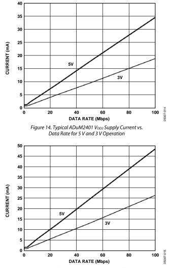
Figure 15. Typical ADuM2402  $V_{DD1}$  or  $V_{DD2}$  Supply Current vs. Data Rate for 5 V and 3 V Operation
