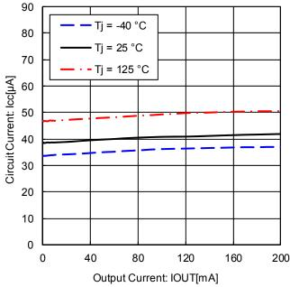
Figure 13. Circuit Current vs. Output Current
