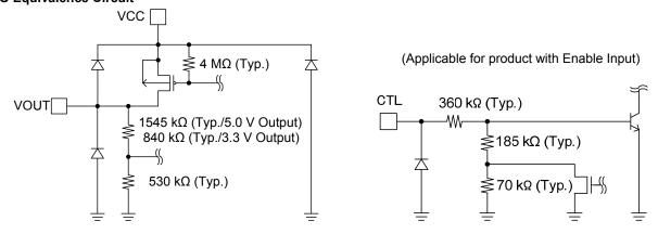
Figure 49. Input / Output Equivalence Circuit
