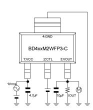
Measurement Setup for Figure 12, 30
