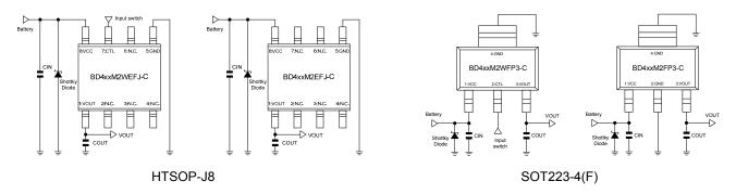
Figure 47. Sample Application Circuit 2
