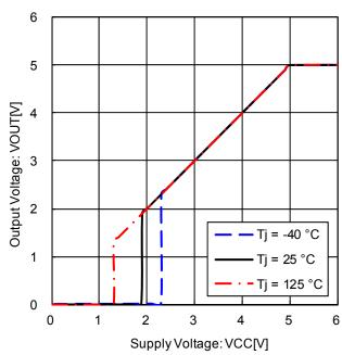
Figure 26. Output Voltage vs. Power Supply Voltage (IOUT = 0 mA)
