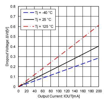
Figure 11. Dropout Voltage (VCC = 3.135 V)
