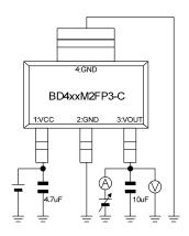
Measurement Setup for Figure 10, 28
