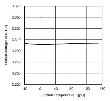
Figure 15. Output Voltage vs. Temperature
