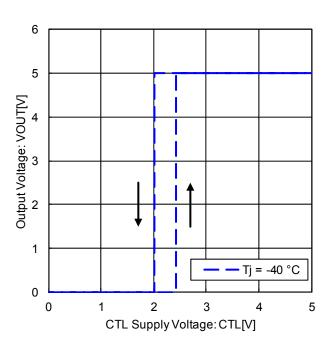
Figure 36. CTL ON / OFF Mode Voltage (Tj = -40 °C)
