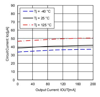
Figure 31. Circuit Current vs. Output Current
