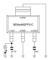
Measurement Setup for Figure 5, 7, 16, Figure 23, 25, 34
