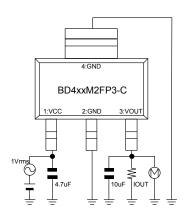
Measurement Setup for Figure 12, 30
