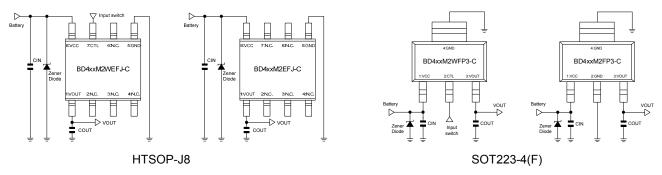
Figure 46. Sample Application Circuit 1
