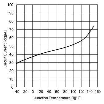
Figure 34. Circuit Current vs. Temperature
