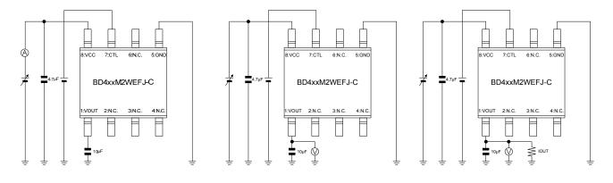
Measurement Setup for Figure 5, 7, 16, 17, 21, Figure 23, 25, 34, 35, 39
