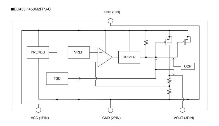
Figure 4. Block Diagrams
