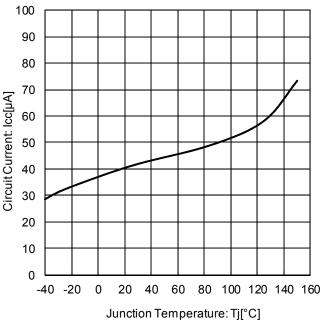
Figure 16. Circuit Current vs. Temperature
