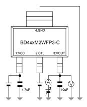
Measurement Setup for Figure 10, 28
