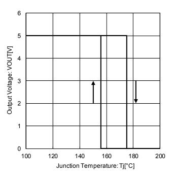
Figure 32. Output Voltage vs. Temperature (Thermal Shut Down)
