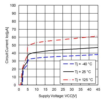
Figure 23. Circuit Current vs. Power Supply Voltage
