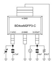
Measurement Setup for Figure 9, 27
