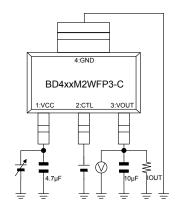
Measurement Setup for Figure 9, 27
