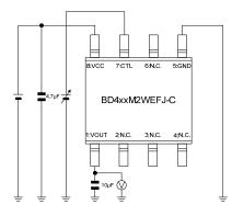
Measurement Setup for Figure 18, 19, 20, Figure 36, 37, 38
