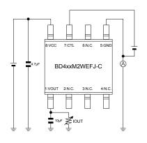
Measurement Setup for Figure 13, 31
