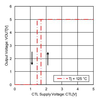
Figure 38. CTL ON / OFF Mode Voltage (Tj = 125 °C)
