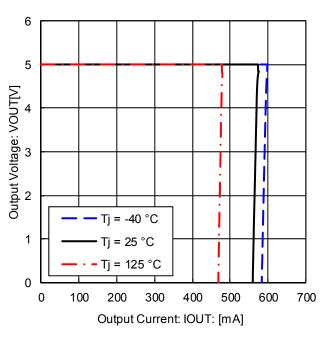
Figure 28. Output Voltage vs. Output Current (Over Current Protection)
