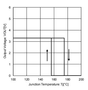
Figure 14. Output Voltage vs. Temperature (Thermal Shut Down)
