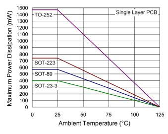
Figure 1. Derating Curves for RT9166/A Packages
