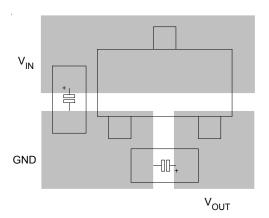
Figure 2. SOT-23-3 Board Layout
