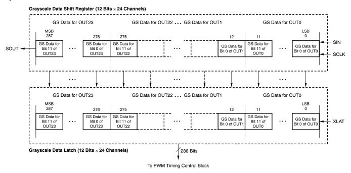
Figure 21. Grayscale Data Shift Register and Latch Configuration
