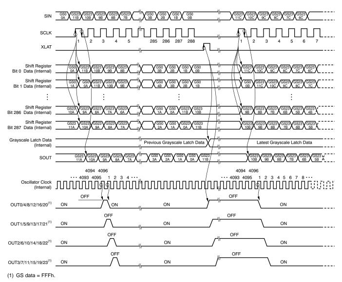
Figure 22. Grayscale Data Write Operation
