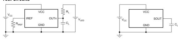
Figure 15. Rise Time and Fall Time Test Circuit for OUTn Figure 16. Rise Time and Fall Time Test Circuit for SOUT
