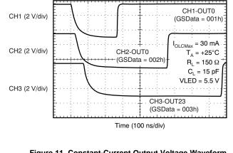
Figure 11. Constant-Current Output Voltage Waveform
