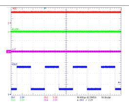
Figure 25. Output Waveform without GS Data Latch Input
