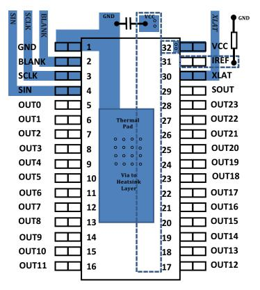
Figure 26. Layout Schematic
