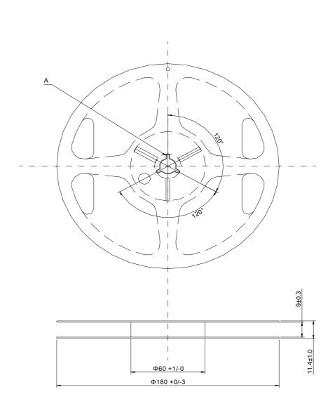
Material:Polystyrene (Conductivity) unit:mm
