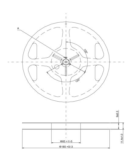
Material:Polystyrene (Conductivity) unit:mm
