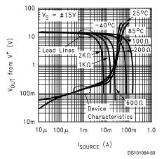
FIGURE 6. Output Sourcing Characteristics with Load Lines
