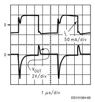
FIGURE 9. V<sub>com</sub> driver performance scope photo
