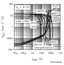
FIGURE 7. Output Sinking Characteristics with Load Lines
