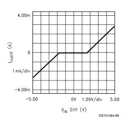
FIGURE 2. Input Stage Current vs Differential Input Voltage
