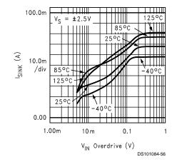
FIGURE 4. Output Short Circuit Sinking Current vs Input Overdrive
