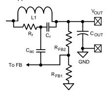
Figure 20. Type III Ripple Circuit
