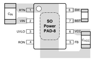
Figure 24. Placement of Bypass Capacitors
