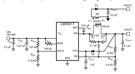
Figure 17. Typical Isolated Application Schematic
