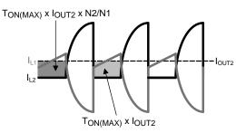
Figure 18. Current Waveforms for C<sub>OUT1</sub> Ripple Calculation
