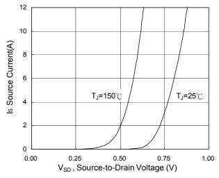
Fig.3 Forward Characteristics Of Reverse
