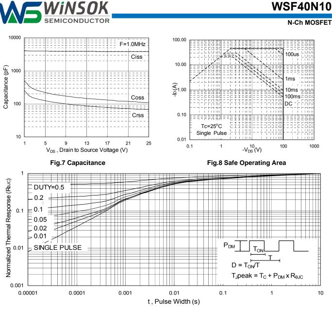
Fig.9 Normalized Maximum Transient Thermal Impedance
