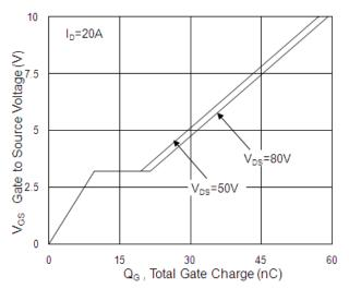
**Fig.4 Gate-Charge Characteristics**
