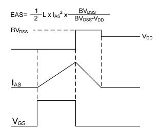
Fig.11 Unclamped Inductive Switching Waveform
