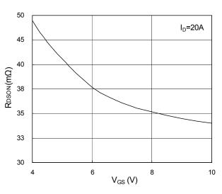
Fig.2 On-Resistance vs. Gate-Source
