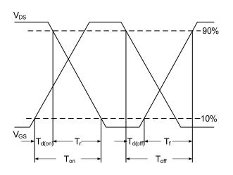
Fig.10 Switching Time Waveform
