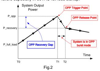
SF5533W can achieve "**Zero OCP/OPP Recovery Gap**" in the whole universal AC input range using SiFirst's proprietary control algorithm.
