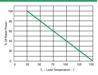
Fig 2.Power Derating Curve
