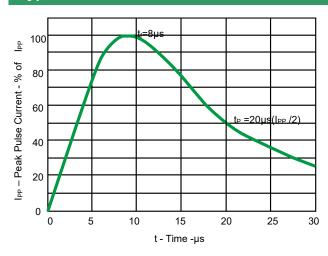
Fig 1.Pulse Waveform
