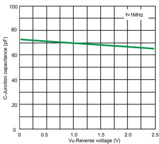
Fig 4. Capacitance vs. Reveres voltage
