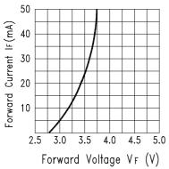
Forward Voltage V<sub>F</sub> (V<sub>j</sub> Fig.2 Forward Current vs. Forward Voltage
