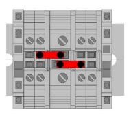
For power supplies, the maximum current carrying capacity of the smallest connected conductors must not be exceeded.
