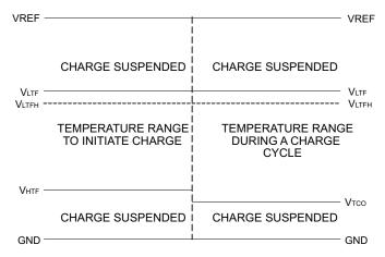
Figure 10. TS Pin, Thermistor Sense Thresholds
