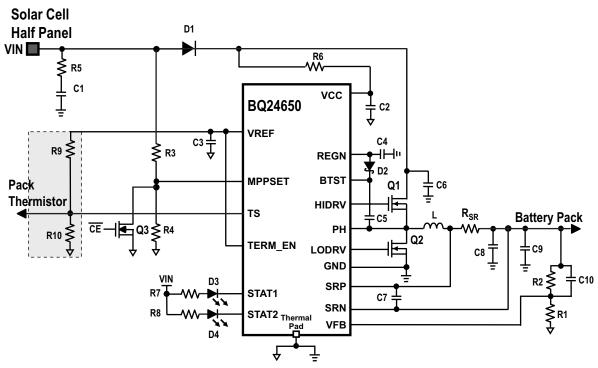
Solar Panel 21 V, MPPT = 18 V, 2-cell,  $I_{CHARGE} = 2$  A,  $I_{PRECHARGE} = I_{TERM} = 0.2$  A,  $TS = 0 - 45^{\circ}C$
