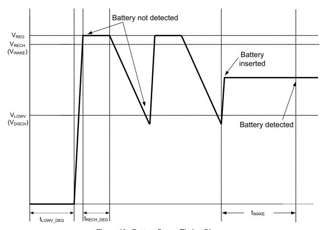
Figure 13. Battery Detect Timing Diagram
