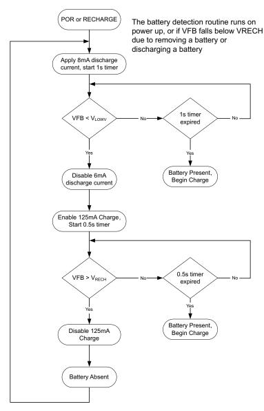
Figure 12. Battery Detection Flowchart
