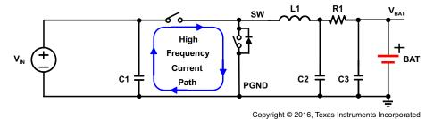
Figure 24. High Frequency Current Path
