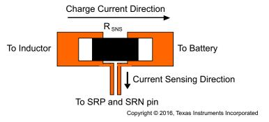
Figure 25. Sensing Resistor PCB Layout
