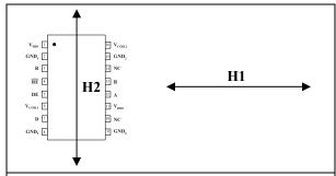
Figure 3. Orientation of External Magnetic Field
