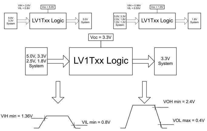
Figure 1. Switching Thresholds For 1.8-V to 3.3-V Translation
