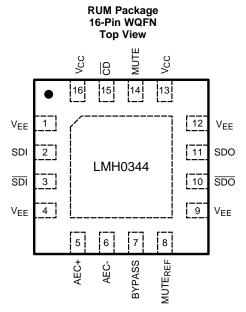
The exposed die attach pad is a negative electrical terminal for this device. It should be connected to the negative power supply voltage.
