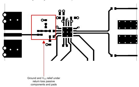
Figure 6. LMH0344EVM Top Etch Layout Example
