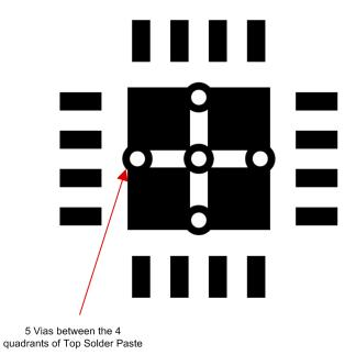
Figure 7. LMH0344EVM Top Solder Paste Mask
