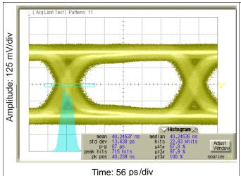
Figure 4. Serial Data Output After Equalizing 100m of Belden 1694A 2.97-Gbps PRBS10
