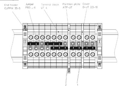
Depending on the separating plate between directly facing plug-in bridges, the rated voltages reduces to
