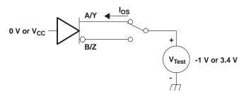
Figure 4. Driver Short-Circuit Test Circuit
