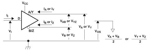
Figure 1. Driver Voltage and Current Definitions
