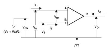
**Figure 9. Receiver Voltage and Current Definitions**
