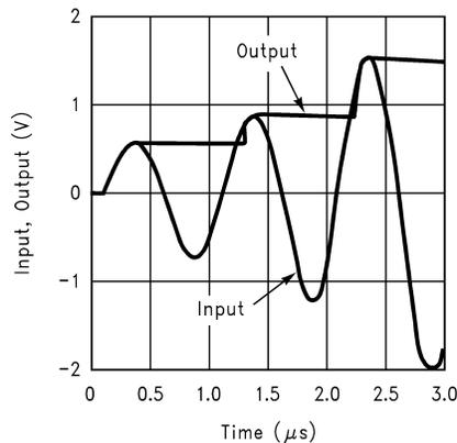
Figure 33. Circuit's Performance With a 1MHz Sinusoidal Input
