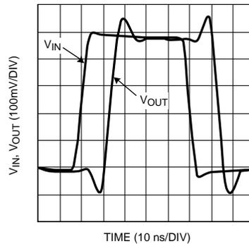
Figure 29. Delay Circuit Response to 0.5V Pulse
