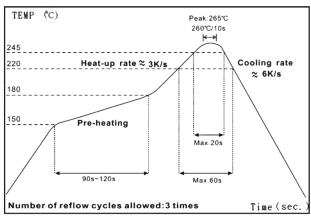
**IR Reflow Soldering**
