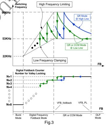
■ At light loading conditions (FB voltage is below VFB\_foldback), the IC works in "Digital Frequency Foldback" mode. The system frequency is limited between "High Frequency Limiting" and "Low Frequency Clamping", as shown with the dashed line in Fig.3. In "Digital Frequency Foldback"
