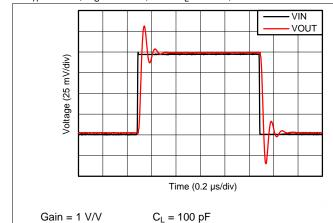
Figure 13. Small-Signal Step Response (100 mV)
