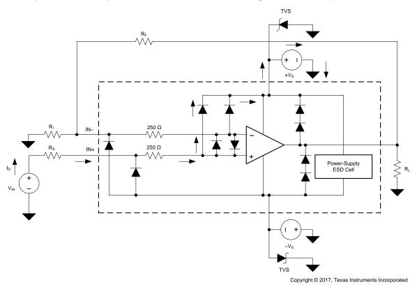
Figure 32. Equivalent Internal ESD Circuitry Relative to a Typical Circuit Application
