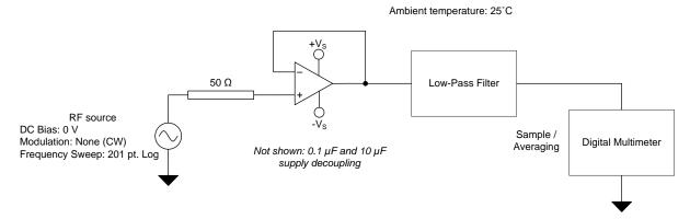
Figure 34. EMIRR IN+ Test Configuration Schematic
