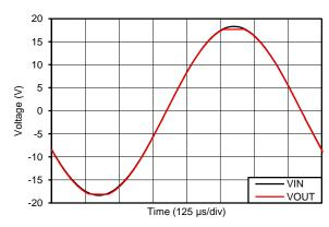
Figure 31. Output Waveform Devoid of Phase Reversal During an Input Overdrive Condition
