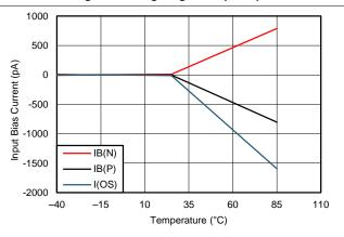
Figure 18.  $I_B$  and  $I_{OS}$  vs Temperature
