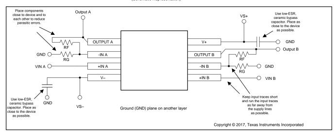
Figure 42. Operational Amplifier Board Layout for Noninverting Configuration
