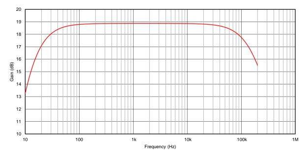
Figure 37. Frequency Response of the Preamplifier Circuit for a 8-nF Piezo Element
