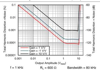
Figure 9. THD+N Ratio vs Output Amplitude
