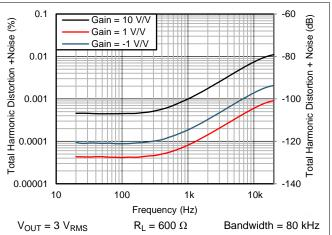
Figure 7. THD+N Ratio vs Frequency
