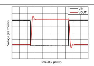
Gain = -1 V/V  $C_L = 100 \text{ pF}$
