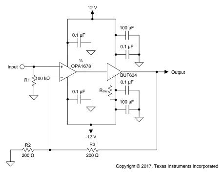
Figure 40. Composite Headphone Amplifier (Single-Channel Shown)
