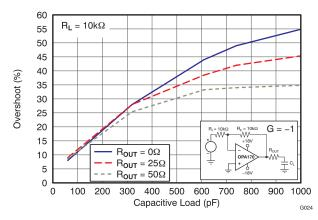
Figure 39. Small-Signal Overshoot versus Capacitive Load (100mV Output Step, G = -1)
