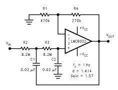
Figure 32. 1 Hz Low-Pass Filter (Maximally Flat, Dual Supply Only)
