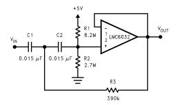
Figure 1. 10 Hz High-Pass Filter
