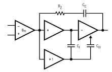
Figure 15. LMC6032 Circuit Topology (Each Amplifier)
