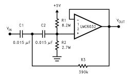
$$\begin{split} &f_c = 10 \text{ Hz} \\ &d = 0.895 \\ &Gain = 1 \\ &2 \text{ dB passband ripple} \end{split}$$
