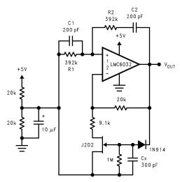
Oscillator frequency is determined by R1, R2, C1, and C2:  $f_{OSC} = 1/2\pi RC$
