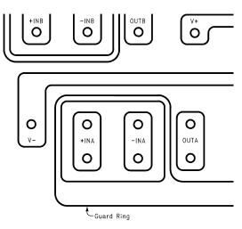
Figure 19. Example of Guard Ring in P.C. Board Layout
