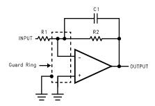
Figure 20. Inverting Amplifier Guard Ring Connections
