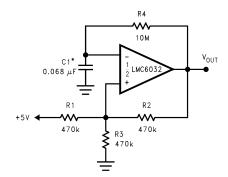
Figure 29. 1 Hz Square-Wave Oscillator
