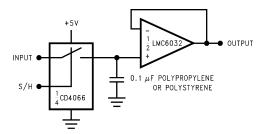
Figure 28. Low-Leakage Sample-and-Hold
