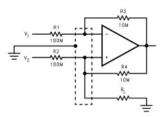
Figure 23. Howland Current Pump Guard Ring Connections
