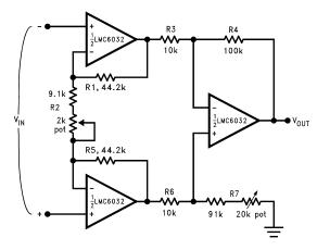
Figure 26. Instrumentation Amplifier
