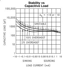
Avoid resistive loads of less than  $500\Omega$ , as they may cause instability. Figure 14.
