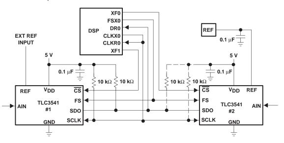
Figure 23. Typical ADC Interface to a TMS320 DSP
