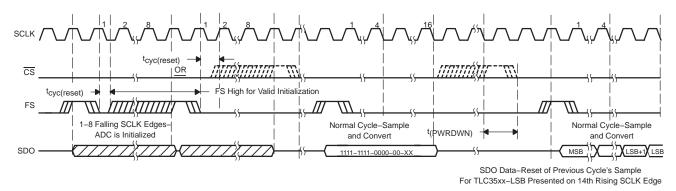
Figure 14. TLC3541/45 Initialization Timing
