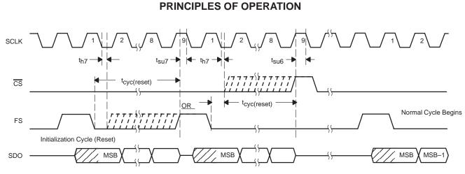
Figure 21. Critical Timing: Initialization Cycle (TLC3541 Only)
