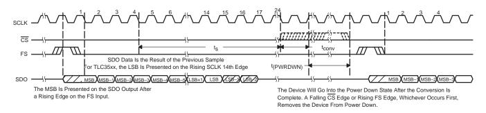
Figure 17. DSP Cycle Timing Using FS Only (or Using Both CS and FS for TLC3541)
