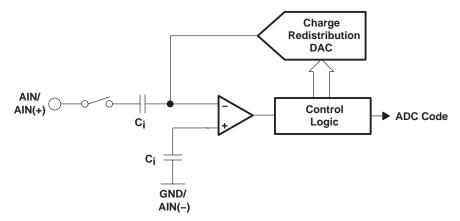
Figure 22. Simplified SAR Circuit
