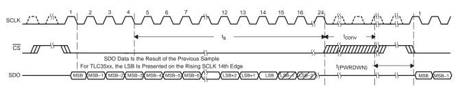
Figure 15. SPI Cycle TIming Using the CS Input (FS = 1 for TLC3541)
