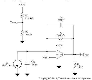
Figure 34. Single-Supply Photodiode Amplifier Circuit
