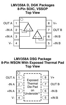
(1) Connect thermal pad to V-
