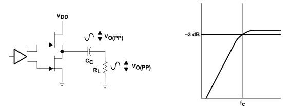
Figure 24. Single-Ended Configuration and Frequency Response
