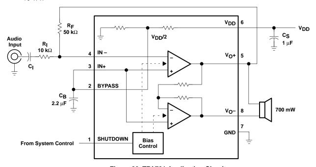
Figure 26. TPA701 Application Circuit
