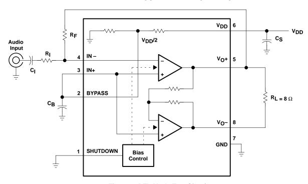
Figure 1. BTL Mode Test Circuit
