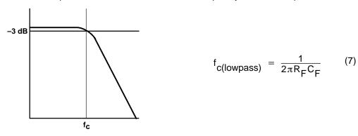
For example, if  $R_F$  is 100 k $\Omega$  and  $C_F$  is 5 pF, then  $f_{co}$  is 318 kHz, which is well outside of audio range.
