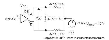
Figure 12. Driver V<sub>OD</sub> With Common-Mode Loading Test Circuit
