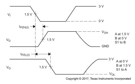
Figure 21. Receiver Enable Time From Standby (Driver Disabled)
