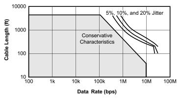
Figure 26. Cable Length vs Data Rate Characteristic
