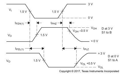
Figure 20. Receiver Enable and Disable Time Test Circuit and Voltage Waveforms With Drivers Enabled
