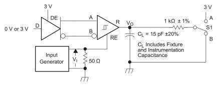
Generator: PRR = 500 kHz, 50% Duty Cycle,  $t_r$  <6 ns,  $t_f$  <6 ns,  $t_o$  = 50  $\Omega$
