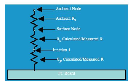
Figure 30. PCB Thermal Resistances
