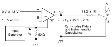
Generator: PRR = 100 kHz, 50% Duty Cycle,  $t_r$  <6 ns,  $t_f$  <6 ns,  $Z_o$  = 50  $\Omega$
