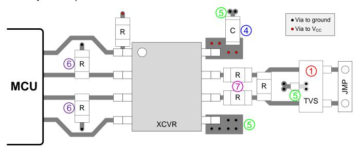
Figure 29. SN65HVD1x Layout Example
