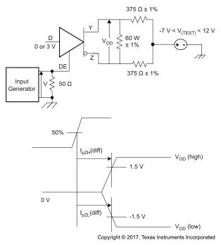
The time  $t_{PZL(x)}$  is the measure from DE to  $V_{OD}(x)$ .  $V_{OD}$  is valid when it is greater than 1.5 V.
