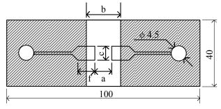
Material: Glass epoxy resin Board thickness: 1.6mm Copper foil thickness: 35µm 2000 : represents a resist pattern.
