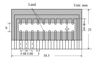
Material: Glass epoxy resin Board thickness: 1.6mm Copper foil thickness:35 μm
