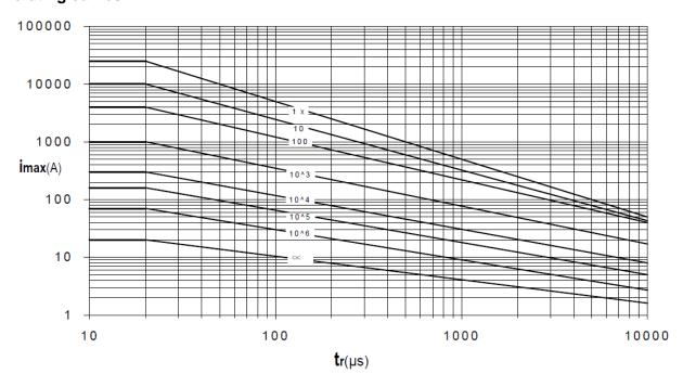
Metal oxide varistor B72232M0461K121V58
